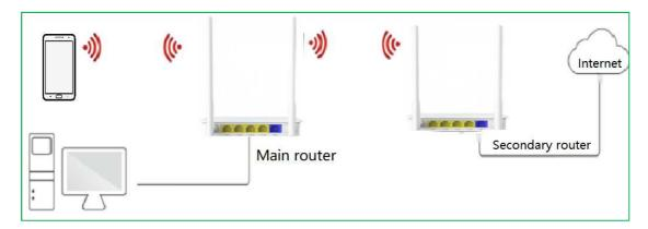
Please note: The secondary router does not need to be connected to the WAN port network cable.
