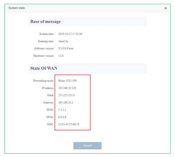
**Note:** If you use the Repeater (Client+AP) mode, after the relay is completed, the IP of the router is issued by the superior. At this time, if you want to login to the management interface of WR138G, you need to set a static IP on the computer. The operation is as follows:
